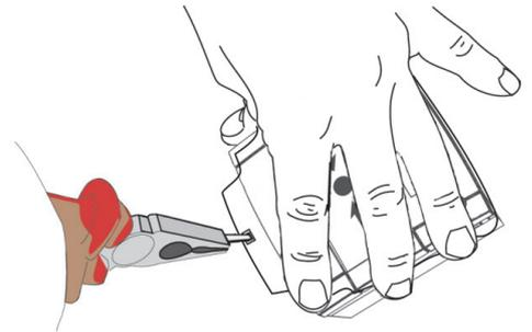
Fig . 4 Using wire cutters, trim the excess from the breakable seal ensuring the tooth remains to hold the hinged cover in position. Fitting cover seal to other classes of call point.
