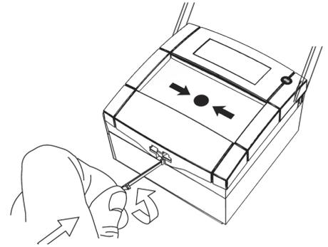
Fig. 3 Feed the other end of the seal through the hole located in the bottom of the hinged cover. Using pliers carefully pull the seal taut and press the hinged cover back to engage the tooth.
